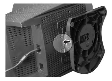
**4** While pressing in the latch, slide the base toward the back of the monitor, then remove the base.
